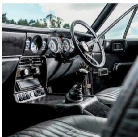
Quad cam V8 came late to the DBS following development problems. Inside, the steering wheel now connects to a nicely weighted power-assisted system
