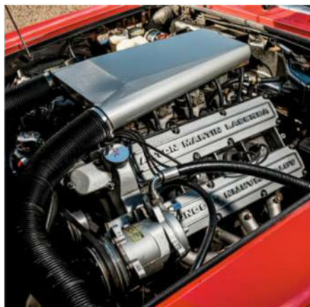
Behind the blanked-off snout lies the Vantage V8 with big valves, high lift cams and raised compression. Owner Alan Medland's advice is to drive it hard, not pootle around
